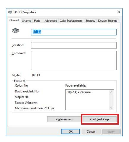
If there is a test page printed by the printer, it means that the Driver's Installation has been finished.
