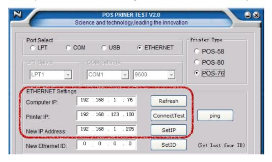
Such as If the user current computer(or POS machine) IP address is 192.168.1.76, but the printer actual IP address is 192.168.123.100, the network segment is 192.168.1, you must modify the same segment as 192.168.1;
